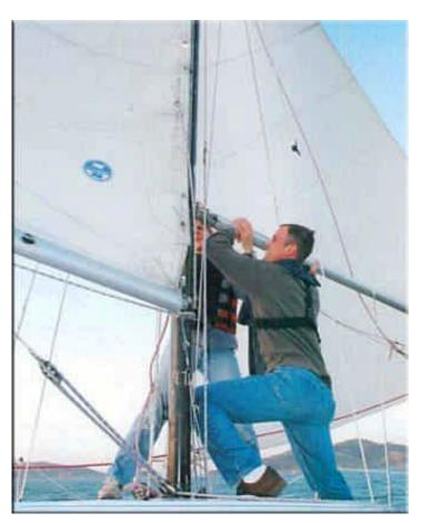
tighten the uppers a little at a time to get their tensions equal and firm. Now adjust the lowers so the forward and rear are firm and balanced. On most boats, the forwards should be a little tighter than the rear.
